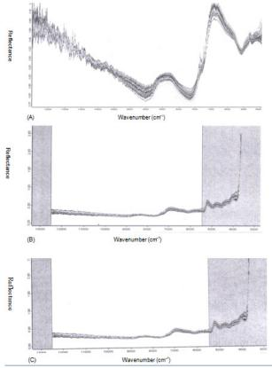
Figure 1. (A) Typical FT-NIR reflectance (log1/R) spectra obtained from Safflower seed samples (B) effect of straight line subtraction spectral preprocessing on original spectra of Safflower seed (C) effect of constant offset elimination spectral preprocessing on original spectra of Safflower seed
